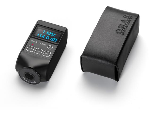
Sound pressure level: 94 dB or 114 dB Frequency: 250 Hz or 1 kHz ANSI: S1.40 IEC: 60942 class 1 The GRAS 42AG Multifunction Sound Calibrator is a portable, battery-operated precision microphone calibrator. The calibrator can be used directly on 1" microphones. Adapters for calibrating 1/2" (factory mounted), 1/4" and 1/8" microphones are included.
